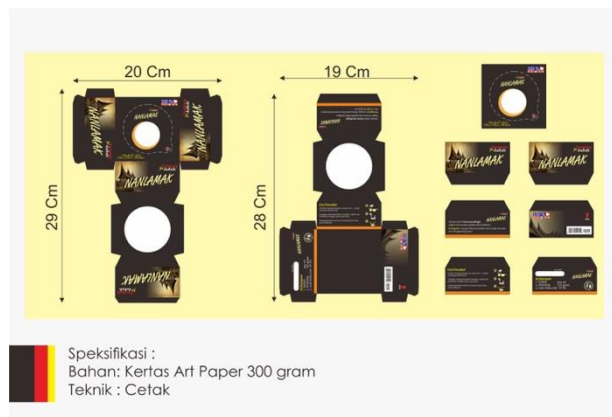
Figure 8. Paper packaging specifications
