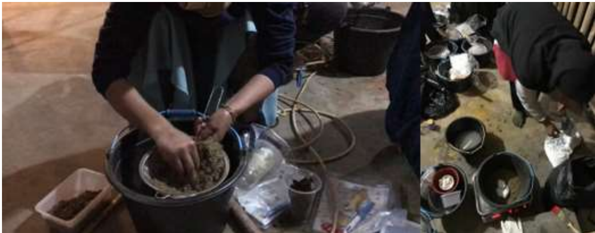
Figure 3. (a) The process of skimming the texture of dried cow dung; (b). The mixing process of the dried cow dung into solid-textured material. (Photos by: PP-PBL ITB)
