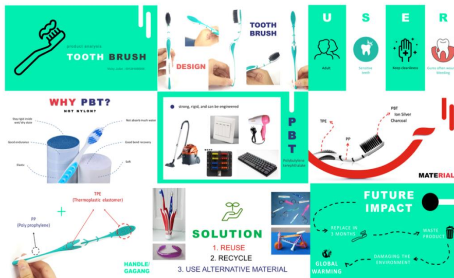
Figure 2. Analysis of plastic application to toothbrush design
